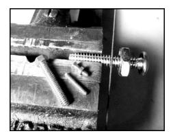
Unscrewing the nut over the freshly cut end of the bolt reforms any of the threads that may have become distorted and knocks off any burrs. Gripping the bolt by the piece to be sawed off localizes any crushing damage to the piece that you'll be throwing away.
