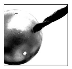
When you drill a hole, there's usually a burr produced on the underside of the metal. Typically you would then file or sand
